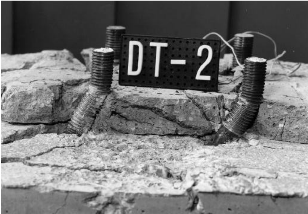
Figure 2.4.10 One of the tested specimens loaded by a combination of shear force and tensile force.
